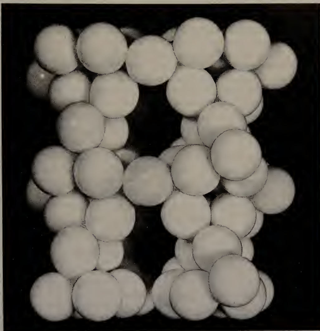
Figure 5-4 Model of a zeolite (edingtonite) showing the channels in the structure. The spheres represent oxygen atoms. The Si and Al atoms lie at the centers of O_4 tetrahedra and cannot be seen. Such a tetrahedron is most easily recognized at the lower right-hand corner of the model.
