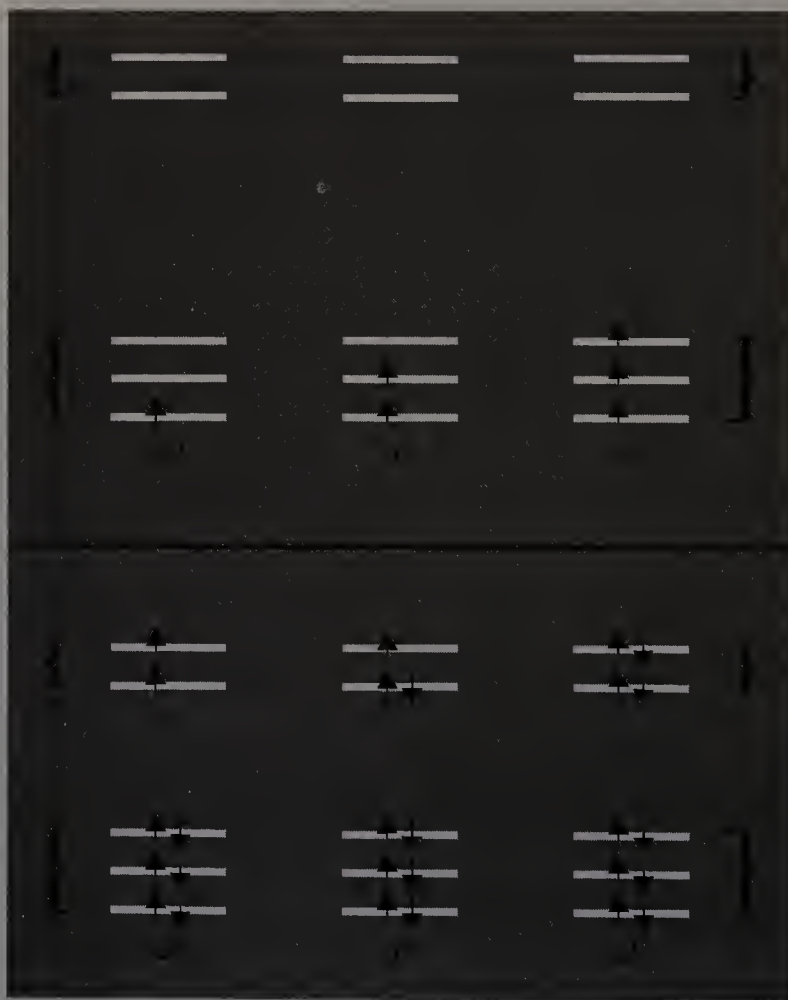
Figure 23-13 Sketches showing the unique ground-state electron configurations for d orbitals in octahedral fields with the d configurations d^1 , d^2 , d^3 , d^8 , d^9 , and d^{10} .
