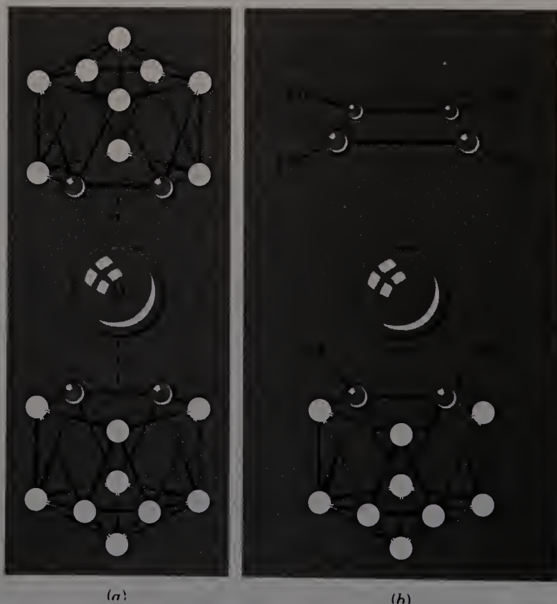
Figure 12-10 (a) The general structure of bis(dicarbollide) metal complexes. (b) An example of a mono(dicarbollide) complex of palladium.
