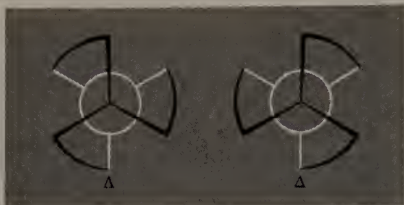
Figure 6-3 Diagrams of tris-chelate complexes showing how the absolute configurations are defined according to twist. The two optical isomers are oriented to show their mirror image relationship. The view for each is along the axis of threefold symmetry.
