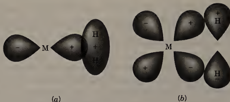
Figure 9-5 The two components of the metal–dihydrogen bond in so-called “side-on” dihydrogen complexes. (a) Donation of electron density from the \sigma -bonding molecular orbital of dihydrogen into an empty \sigma orbital of the metal, and (b) “back-donation” of \pi -electron density from a filled d orbital of the metal into the \sigma^* antibonding orbital of the H—H linkage. Both components of the M—H 2 bond weaken the H—H linkage.
